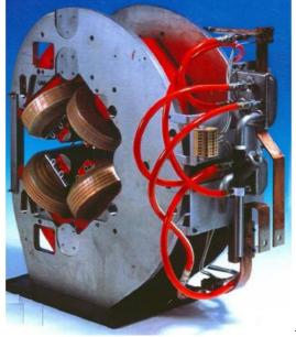
Type: Laminated Yoke -**Ouadrupole** low carbon steel Yoke: Conductor: **OFHC** copper 2 GeV Energy Gradient 20 T/m Magnet Bore Diameter 75 mm Field Quality < 10<sup>-3</sup> Magnetic Length 470 - 230 mm Ampere-Turns per Pole 12800 Current 320 A Conductor Size 9 x 6.8 mm<sup>2</sup> Coolant Hole Diam. 4.6 mm 8.6 - 5.4 KW Power Water Circuits per Magnet 4 Magnet Weight 1400 - 840 Kg
