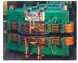
Type: **Laminated Yoke** - Dipole Yoke: Low carbon steel Conductor: **OFHC** copper Energy 2 GeV Maximum field in center 1.455 T Bending radius 5500 m Type of winding double pancake Nominal current 1,950 A
